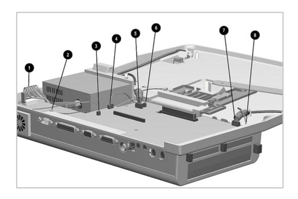
Figure 7-18. Disconnecting and Removing the Main Board Cables
